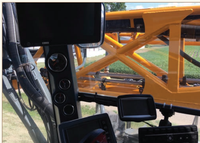
When spray booms are folded, it makes it difficult to see if anything is approaching your rig. Adding monitors, screens, and computers in the cab to improve sprayer control further obstructs the driver's view (bottom).
