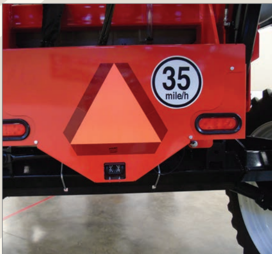
The camera on this sprayer is mounted just below the slow-moving sign. Using the touch screen and rear camera option, operators can easily view what is directly behind them while traveling or backing up.
